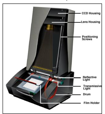
This is sort of like an upside down enlarger. Where the image is transmitted onto the CCD array. With 4"x5" film the lens will be closer to the CCD while 35mm the lens will be closer to the film. Since the CCD is a fixed number of pixels, the farther away the lens is, the more pixels per inch of resolution we will
