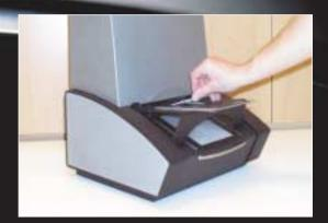
2. When the slide mount is in the holder scanning can be performed as usual. Select "35 mm Slide" in the Colorflex frame menu.
