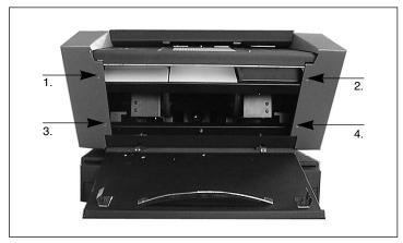
Figure 10: Front screws for securing the side plates.
