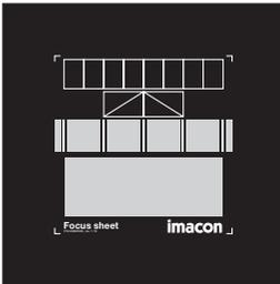
2. Load the sheet into the 6 x 6 original holder with the lines pointing towards the scanner (vertically). Place the sheet as straight as possible. Use the scanner's light table grid and the corners marked on the sheet to help align it.
