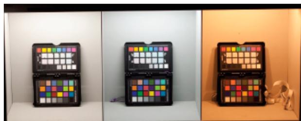
One simple way is a light box. Commercial units like on the right, are available or you can make your own. Above is a light box showing Daylight, Fluorescent and tungsten light sources. You can see the effect of the different light sources on the Color Checker. I made the above light box out of cardboard banker boxes with 3 different light sources. You can
