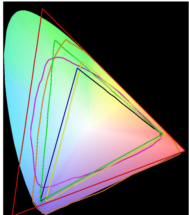
In this representation, the multicolored inverted horseshoe represents what the human eye can see. The large red triangle is the Pro Photo Working space. The Green triangle is the Adobe 1998 working space and the Dark Blue triangle is the sRGB working space. The working spaces are used in Photoshop to determine how much area to spread out our image data into. In order to know which space is best for us we need to look further at
