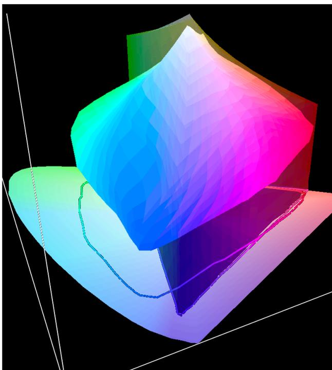
Notice the large mass of blue/green info that the printer can print but the monitor cannot see, if we are using the iMac display. We could use the sRGB working space and the monitor display would cover it. But we would be clipping off the more brilliant
