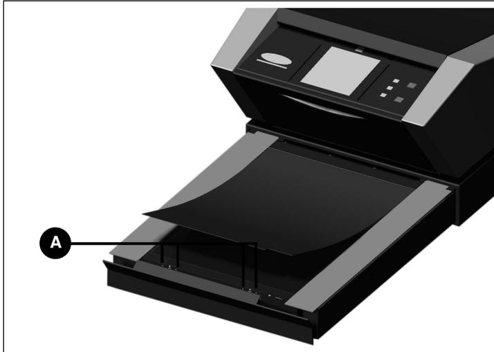
*Figure 5: Replacing the electrostatic plate. The contact pins (A) must enter the holes in the electrostatic plate.*
