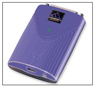
At the time Imacon introduced the P-2 to P-3 upgrade we shipped all new scanners with the 2nd Wave adapter. Success was very mixed and what we didn't know then was a power issue. Remember I said the SCSI chain gets power from the card. These devices get their power from the Firewire connection. Most of the time it was not enough power to made it down the SCSI chain to the terminator.
